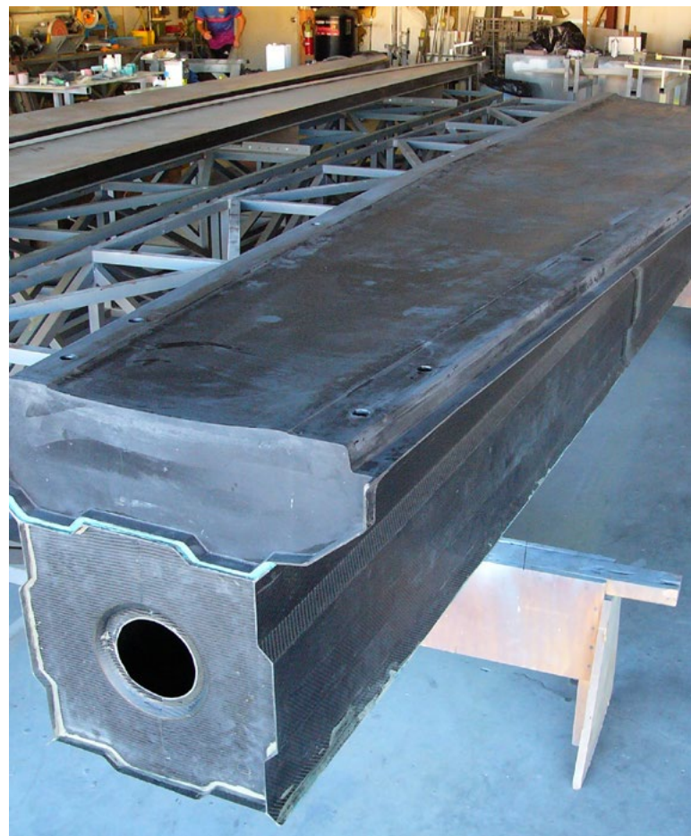
Picture 3 – carbon fiber mold for the outer wing
