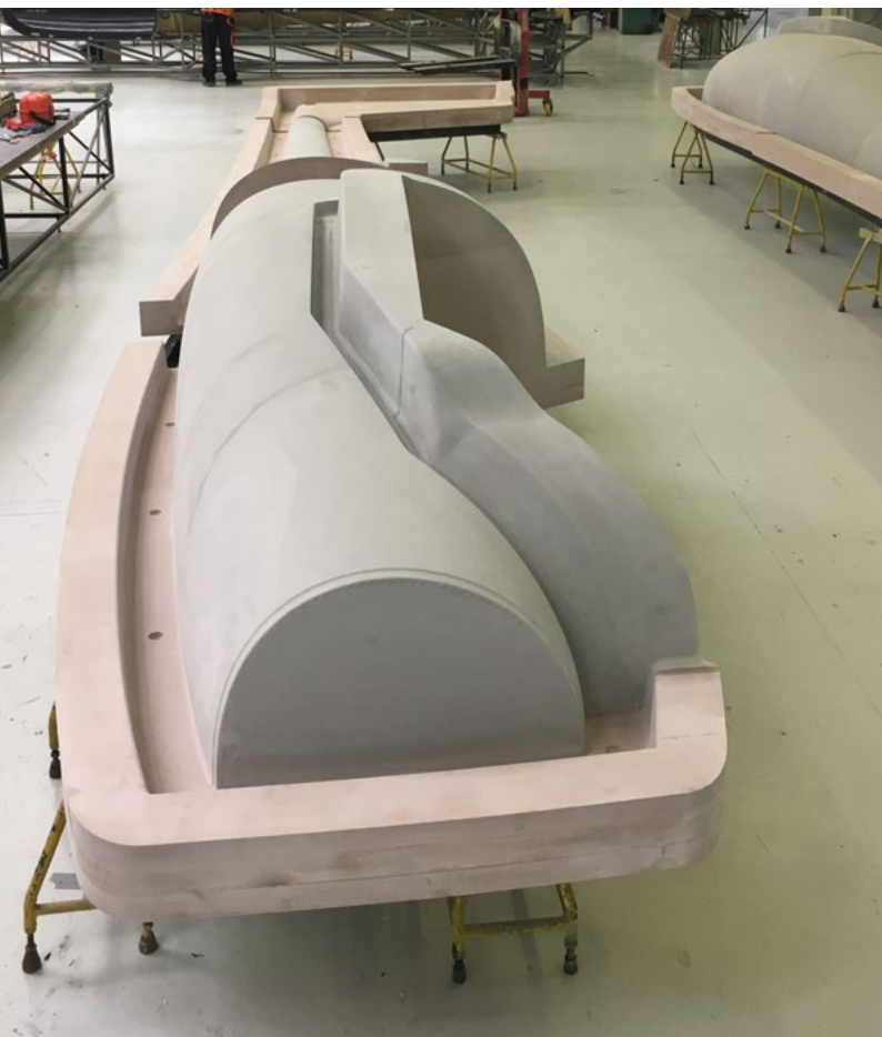
Picture 2 – fuselage master model
